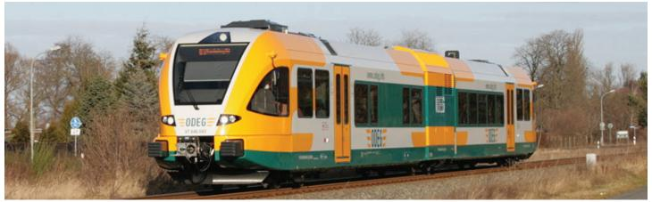
Non-electrified regional rail/commuter systems in Europe that carry less than 500 passengers on the busiest peak hour trains use diesel multiple units (DMUs) almost exclusively. In contrast, most new U.S. commuter rail systems carry less than 10,000 passengers per day use locomotive-hauled trains, with only a handful of exceptions. These systems generally serve less than 500 passengers on their busiest peak hour trains.
