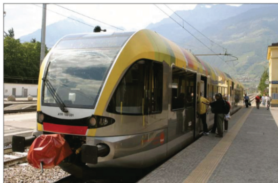
Level boarding at low platforms speeds Val Venosta trains. Despite 2.9% grades, trains now average over 30 mph.
