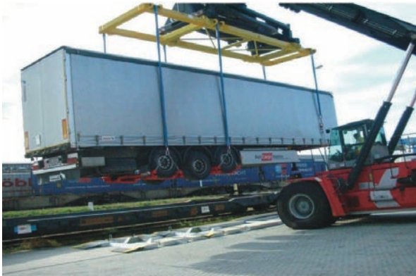
ISU technology used in Austria for quickly loading & unloading trailers. (Source: Rail Cargo Austria)
