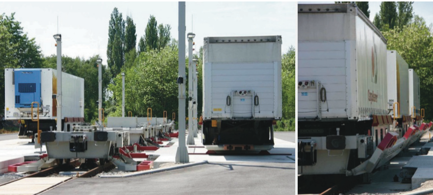
"CargoBeamer" is an innovative, automated European terminal that slides trailers on/off freight cars for quick loading & unloading of intermodal traffic. (Source: CargoBeamer)
