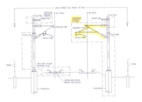
Figure 3-1 Typical 2x25 kV Electrification System
